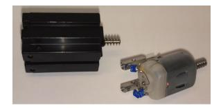
The motor itself consists of two permanent magnets in a case which establishes a magnetic field between them.
