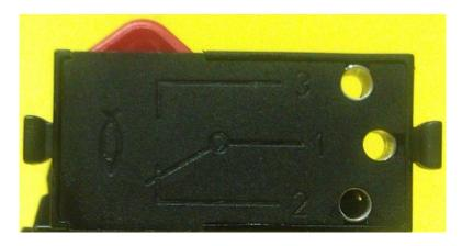
For this exercise we will connect the wire to holes 1 and 3. Connect the red wire to hole 1 and the green wire to hole 3. It should look similar to the picture below.
