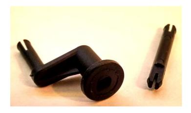
Line up the clip end of the axle with the opening in the crank shaft. Insert the shaft into the crank shaft. It will look like the picture below.
