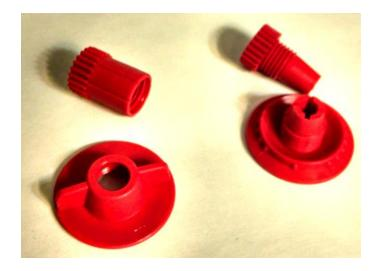
They consist of a threaded part that has separations in it. As the tapered cap is threaded onto the collet the sections of the collet squeeze together and clamp onto the shaft passing through the center. When the collet is lose the shaft is free to pass in and out. When the cap is tightened the movement ends and the shaft is caught in position. In the example below a collet is used to hold a gear in position on a shaft.
