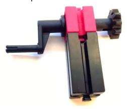
Find the base plate and place that on your table. Slide the end of the block 30 into the first short groove on the plate. Below are two views of the assembly so far.
