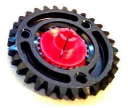
Now insert the clip axle in the center of the flat hub collet. The table will keep the axle from going all the way through the collet.
