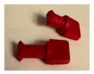
The rivets are shaped so they only pass through the shape in one position and then are rotated to make removing the rivet difficult.
