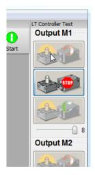
Click on the top icon which is the motor counterclockwise direction. You should hear your motor begin to turn. The top icon will be true color and the stop button greyed out. To stop the motor, left click on the STOP button. The motor should stop and the STOP button will be bright once more.
