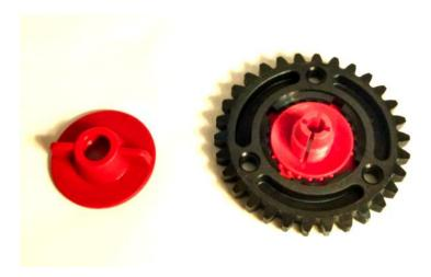
Notice the collet has notches on the outside to help the gear connect with the collet.
