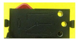
With the cover removed the internal components are visible. The number 1 connection is the middle contact. You can see that it is in contact with the contact with the number 2 connection making the 1 & 2 normally closed and the 1 & 3 normally open. When the button is pushed the connection between 1 and 2 is opened and the connection between 1 and 3 is closed. This is a temporary connection as the spring will return the switch to its normal position as soon as the pressure is released.
