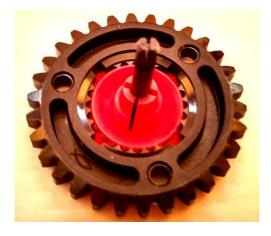
Place the hub nut over the axle and tighten the nut so it is tight and the axle will not move. Tighten it only with your fingers to prevent damage. Engineers call this finger tight.
