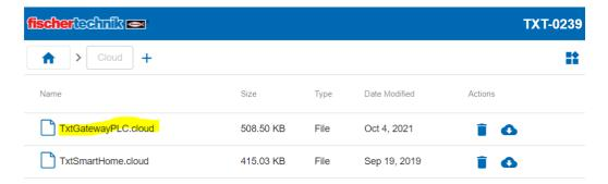
Connect the TXT controller with the fischertechnik Cloud as described in the didactic material (<a href="https://www.fischertechnik.de/de-de/service/elearning/simulieren/lernfabrik-24v">https://www.fischertechnik.de/de-de/service/elearning/simulieren/lernfabrik-24v</a>). Only if the pairing is successful the program in the folder Cloud can be selected on the TXT controller.
