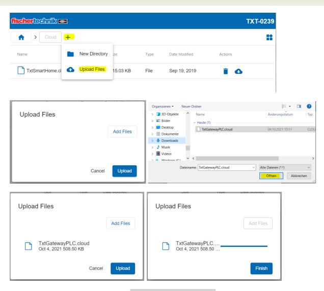
Download and save the program **TxtGatewayPLC.cloud** on the computer as described above. The dowloaded program must be copied to the "Cloud" folder on the TXT controller.
