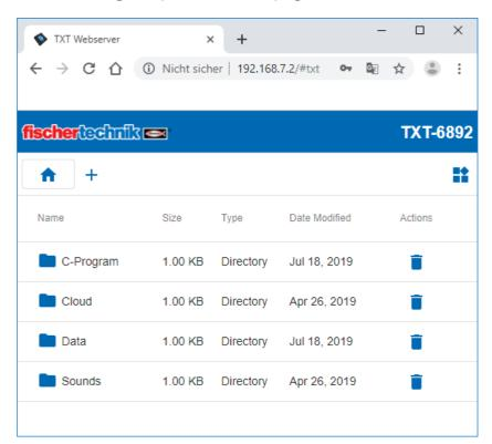
To copy C programs to the TXT controller, change to the directory "Cloud" by clicking on it with the mouse. In this directory fischertechnik cloud C programs are stored on the TXT controller. Files can be deleted using the Recycle Bin icon or added via the + icon. If you click on +, a dialog box opens in which you can select files on the computer with "Upload files" and add them with "Add Files". If one or more files have been selected, they are uploaded to the TXT controller with "Finish".
