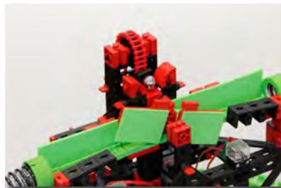
After the ball has been knocked off the magnetic ball holder, it rolls into the automatic cross-over, which routes the balls alternately to the left and right.
