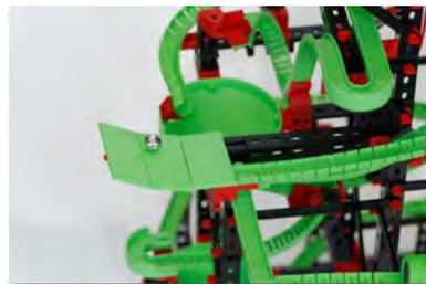
The balls roll from the flex-rail onto the quarter pipe, which consists of three construction plates. It is inclined slightly upward and to the side so that the balls drop into the rotary funnel after changing direction.
