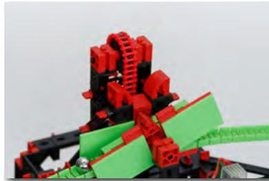
After the ball has been knocked off the magnetic ball holder it rolls into the automatic cross-over which routes all incoming balls alternately to the left and right.
