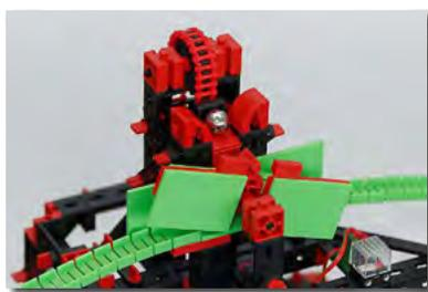
As soon as a ball holder passes by a steel ball in the model's magazine, it is attracted by the magnet and transported to the top. At the top the ball is pushed off and rolls through the obstacle course.
