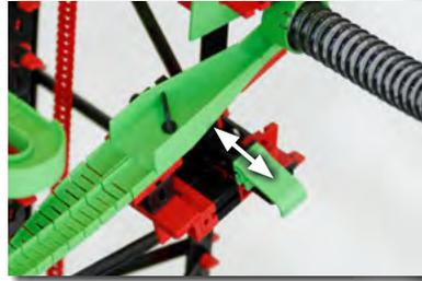
The switch with switch lever are used to determine the direction of the course.
