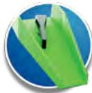
A lever is attached in the middle of the **cross-over** to guide the balls alternately to the flex-rail attached on the right or left.
