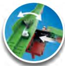
The **cross-over locking lever** is installed in the sub-frame of the cross-over. It is driven by a rack and pinion with locking mechanism, enabling manual adjustment of the cross-over.
