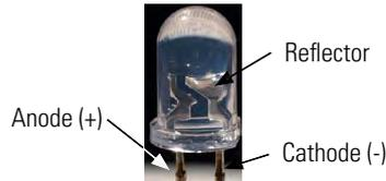
**Important!** The LEDs used in the construction set are built into a bulb module. Here it is necessary to observe the polarity as described in the assembly instructions.
