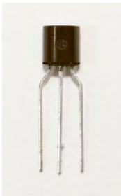
■ The transistor, also called a bipolar transistor, is also an electronic component. It is used for switching and amplifying electrical signals. Transistors are the most important constituents in electronic circuits. Transistors have a special significance in integrated circuits. The name transistor was derived from its function. If the resistance of one semi-conductor layer changes, the resistance of the other layer also changes. The concept "transfer resistor" was shortened to "transistor".
