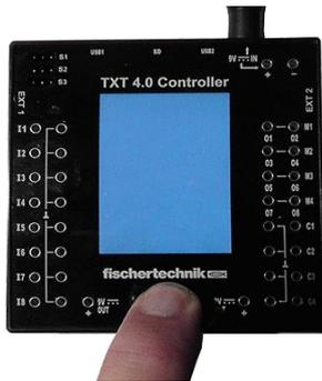
Press the ON/OFF button for approx. 4 seconds, until the display switches on. The TXT 4.0 Controller will boot up.
