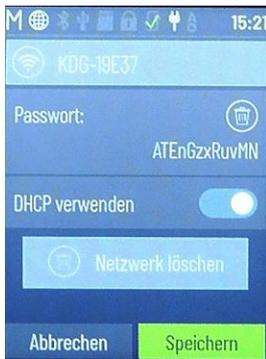
Then, the TXT Controller needs to be connected to the WiFi router. To do so, press “WiFi”. The available networks are displayed in the new window. Activate your network here. The input window will appear for you to enter your router password. This is provided in the documents for your router. After entering it, end the setting by pressing “Save”.
