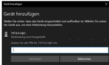
You now need to enter the PIN for the TXT 4.0 Controller in the connection window. This is found on the Controller display as the "Coupling code" under Settings – Network – Bluetooth
