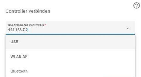
The IP address “192.168.7.2” of the TXT 4.0 Controller is selected and displayed automatically.
