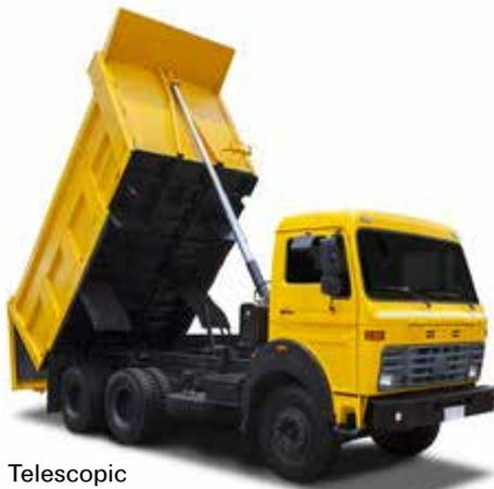
Telescopic cylinder on a dumper truck
