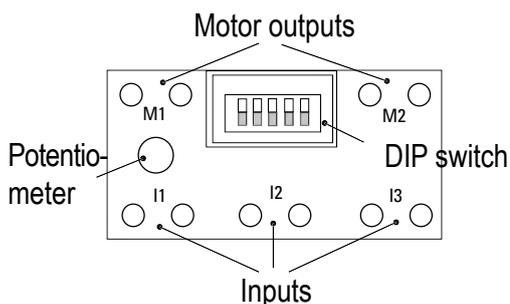
The ROBOTICS module works only when it is connected to a 9 V power supply. For this purpose use the battery tray with a 9 V block battery either as dry cell or rechargeable battery. When connecting ensure that the polarity is correct (red = positive). When the module is supplied with power correctly, the green LED illuminates.
