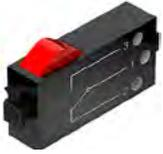
The pushbutton could also be called a touch sensor. Pressing the red button actuates a switch mechanically allowing electricity to flow from contact 1 (middle contact) to contact 3. At the same time the circuit between contacts 1 and 2 is interrupted. So you can use the pushbutton in two different ways:
