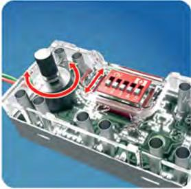
The potentiometer on the ROBOTICS module allows you to control the speed of the two drive motors. When the potentiometer is in the middle position (viewed from above, so that the DIP switch designation is easily legible) both drive motors turn at the same speed propelling the Mini Bot straight ahead. Turning the potentiometer to the left causes it to curve to the left while moving forwards. Turning the potentiometer to the right causes it to curve to the right while moving forwards.
