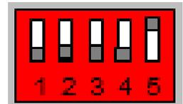
After setting DIP switch 5 to ON and all others to OFF, you can switch on the power supply for the ROBOTICS module on the battery tray. The program last saved is then run through once. To run the program again, it is necessary to switch off the power supply to the ROBOTICS module and then switch it back on.
