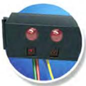
The infrared trail sensor is a digital sensor for identification of a black trail on a white background at a distance of 5 to 30 mm. It consists of two transmitter and receiver elements. For connection you need a digital input on the ROBOTICS module and the 9 Volt power supply (positive and negative poles) on the battery tray.
