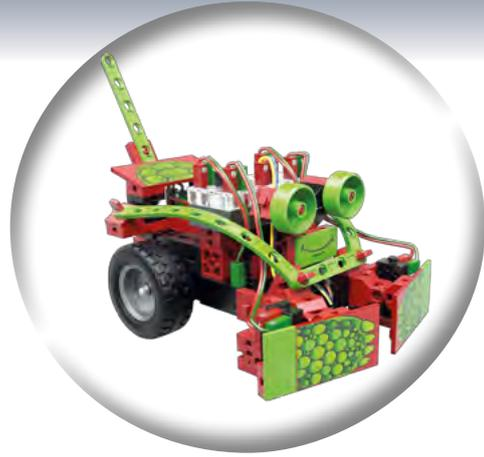
With the ROBOTICS Mini Bots Construction Set you can build one of the Mini Bot models: mobile robot, hindrance detector, trail searcher, hindrance detector with trail sensor or teach-in mobile robot.
