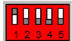
To help you get started the mobile robot model is not initially equipped with sensors. After setting the DIP switches for the mobile robot program as shown above, connecting the power supply on the battery tray and starting the ROBOTICS module program, the two drive motors start turning and the mobile robot moves forwards.
