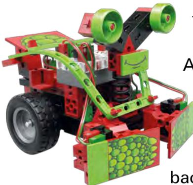
The Mini Bot hindrance detector is equipped with two mini-switches on the two bumpers which serve as sensors. After starting the program the Mini Bot moves straight ahead. It continues this until one of the bumpers touches an obstacle.
