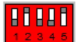
Proceed as follows to have the Mini Bot teach-in mobile robot run along a path continuously. After setting DIP switches 2 and 5 to ON and all others to OFF, you can switch on the power supply for the ROBOTICS
