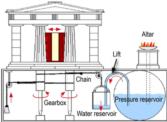
Over 2000 years ago the Greek engineer and inventor Ktesibios built the first machines powered by compressed air, for example, a catapult which used compressed air to hurl shot and spears. Heron of Alexandria built one of the best known compressed air systems, which used the altar fire to generate compressed air to open the huge temple doors, as if by magic.
