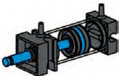
We use pneumatic cylinders to generate motion with air. As a matter of principle we differentiate between "single acting" and "double acting" cylinders. Your Pneumatic Power Construction Set contains three different sizes of pneumatic cylinders with the same "double acting" function.
