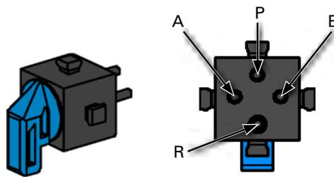
The middle connection P is for the compressed air coming from the compressed air reservoir. The left or right fitting (A or B) guides the compressed air to connection A or connection B on the cylinder. The connection marked R on the bottom of the valve serves to release the air or "relieve" the air pressure. This allows the air returning from the cylinder to escape. Perform the following experiment to see how the valve works.
