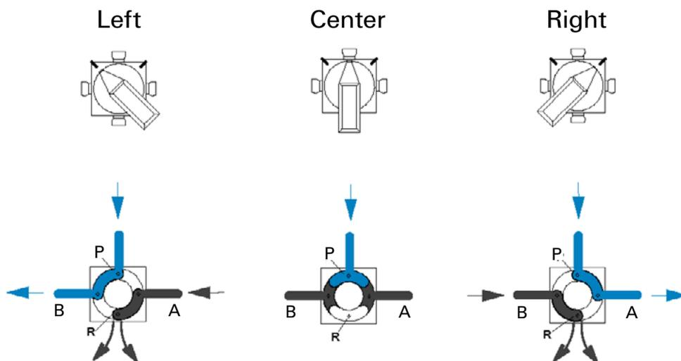
The valve has **four** connections and **three** switch positions (center - left - right). For this reason the valve is called a 4/3-way valve in pneumatic jargon.
