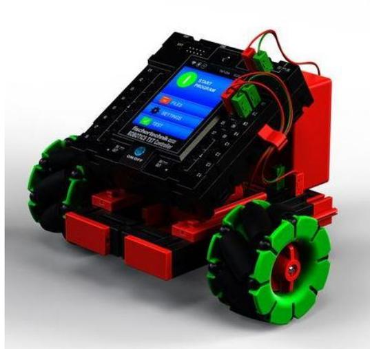
If you have built the model using the building instructions, you have probably already noticed two new components – the Omniwheels and the support wheel.
