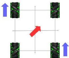
If you want the model to travel diagonally to the right, only 2 motors are required as shown in the image. These will turn in the same direction (to the left) and at the same speed.
