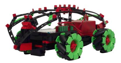
All 4 Omniwheels and the gesture sensor (colour recognition and gesture control), as well as the track sensor, are used in this model.
