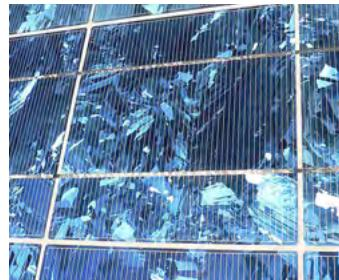
A solar cell or photovoltaic cell is an electrical component, which converts the radiant energy in light (usually sunlight) directly into electric energy. The physical principle of this conversion is called the photovoltaic effect. Solar cells should not be confused with solar collectors, with which the solar power heats up a transfer medium (usually hot water for heating).
