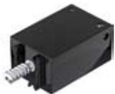
The XS motor is an electric motor, which is exactly as long and high as a fischertechnik building block. In addition, it is very light. This allows it to be installed at locations where there is insufficient space for larger motors. The XS motor is designed for a voltage of nine volts and current input of a maximum of 0.3 amperes.
