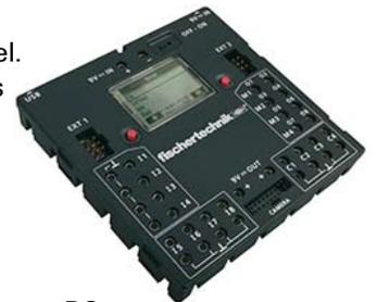
A special treat is the integrated Bluetooth interface. It allows you to connect your PC to the ROBO TX Controller. Or to connect a number of controllers with one another. You can define how the controller interacts with the individual components and what they are to do in detail in the program you write with the ROBO Pro software.
