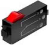
The pushbutton is also called a touch sensor. When the red button is pressed a switch is switched mechanically allowing current to flow from contact 1 (middle contact) to contact 3. Simultaneously the contact between connections 1 and 2 is interrupted. So you can use the pushbutton in two different ways:
