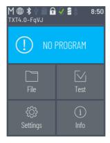
If "NO PROGRAM is displayed after this process is complete, then the error was successfully corrected, and the Controller can be connected to ROBO Pro Coding once again.
