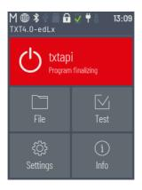
If the TXT 4.0 Controller displays the red button labeled "txtapi" approx one minute after it is switched on for the first time, then a connection cannot be formed with ROBO Pro Coding.
