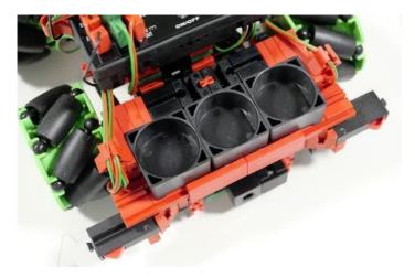
The power supply for the AGV is provided by the fischertechnik battery included in the scope of delivery. It is delivered already charged up, so you can start the AGV directly.
