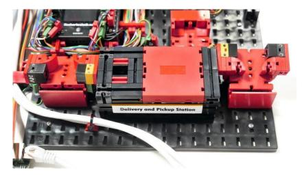
There are three different colors that can be produced by the APS. Stickers are attached for each color that are detected as OK or NOK (not OK) by the quality assurance.
