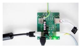
Ensure that all cables are securely connected to the connection boards. Then plug the 24 V power supply and 9 V power supply into an outlet and use the following description with LED 1 and LED 2 to ensure the modules are supplied correctly with power.
