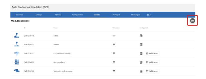
This view also offers the possibility of calibrating modules. Module-specific positions and distances are set in this process. The APS is delivered pre-calibrated; however, the modules may be moved during setup and disassembly. If a module no longer grips the workpiece precisely, you can correct this via the calibration. Instructions for doing so are found at the following link:
