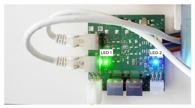
In addition, there are two buttons with LED 2 on each connection board to the power supply. These are used as an emergency stop for the individual module.
