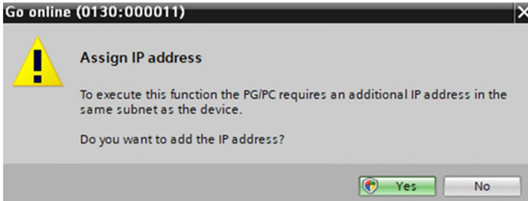
Picture 6 Advanced loading - Assign IP address
