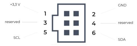
The Combi-sensor can be connected to the EXTI **or** EXT2 port. Example of connection to the TXT 4.0 Controller. <u>Only one Combisensor</u> can be connected to a Single TXT4.0 controller.
