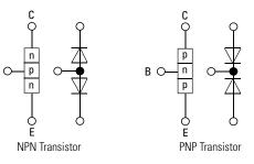
npn and pnp transistors, whereby the letters designate the layer sequence. The middle layer is very thin in comparison to the other two layers. The layers are provided with connections leading out of the housing. The outer layers are called the collector (C) and emitter (E). The middle layer is the base (B). It is the control electrode or the control input for the transistor.
