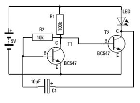
■ Wind power stations and transmitter masts as well radio antenna towers and airplanes have a flashing light to visually signal their position as a safety precaution. Construct the demonstration model of a simple flasher and wire the electrical components as shown in the circuit diagram.
