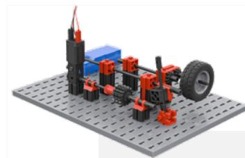
1. The following three-speed manual transmission (with two Z30, two Z20, and two Z10) achieves gear ratios of 1:3, 1:1, and 3:1.
