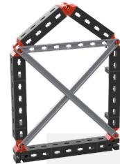
Static determinacy describes the property of a system in which all unknown forces and moments can be calculated solely on the basis of the equilibrium conditions. It is a central concept in statics and characterizes the support of stationary bodies as well as the internal structure of body systems such as half-timberings.
