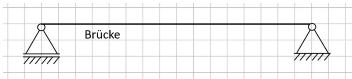
On the left side is a pendulum support, which acts as a single-value bearing for the bridge structure. This bearing can only absorb compressive or tensile forces perpendicular to the bearing. This type of bearing is also called a sliding or loose bearing, as it can move freely in the horizontal direction.
