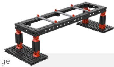
Please note that for these values, half the weight of the bridge must be subtracted from the measured value. In reality, the weight of a bridge is much greater in relation to the traffic or wind loads acting on the structure.
