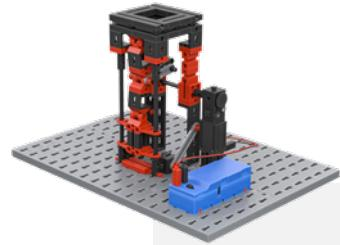
Place objects of different thicknesses under the press, such as paper, modeling clay, or thin pieces of wood, and compare the model with the eccentric press.
